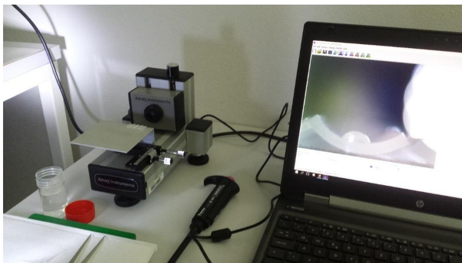
Figure 3.3: WCA equipment and measurements.
