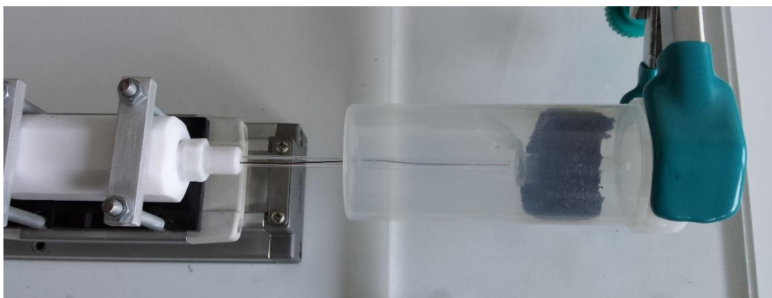
Figure 4.17: Dynamic horizontal CAP treatment with argon atmosphere.
