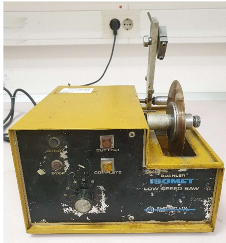
Figure 3.12: Precision sectioning saw with a diamond blade – BUEHLER IsoMet Low Speed Saw.
