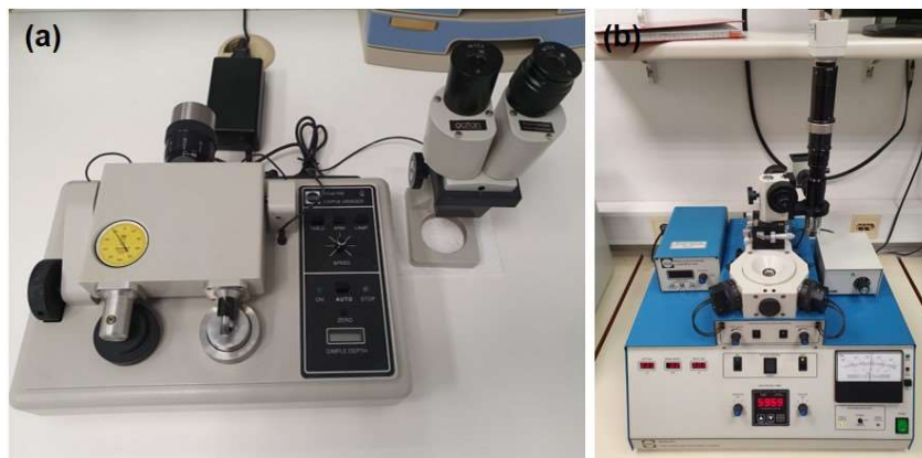
Figure 3.14: (a) Dimple grinder – model 656 and (b) Precision Ion Polishing System (PIPS) – Gatan.
