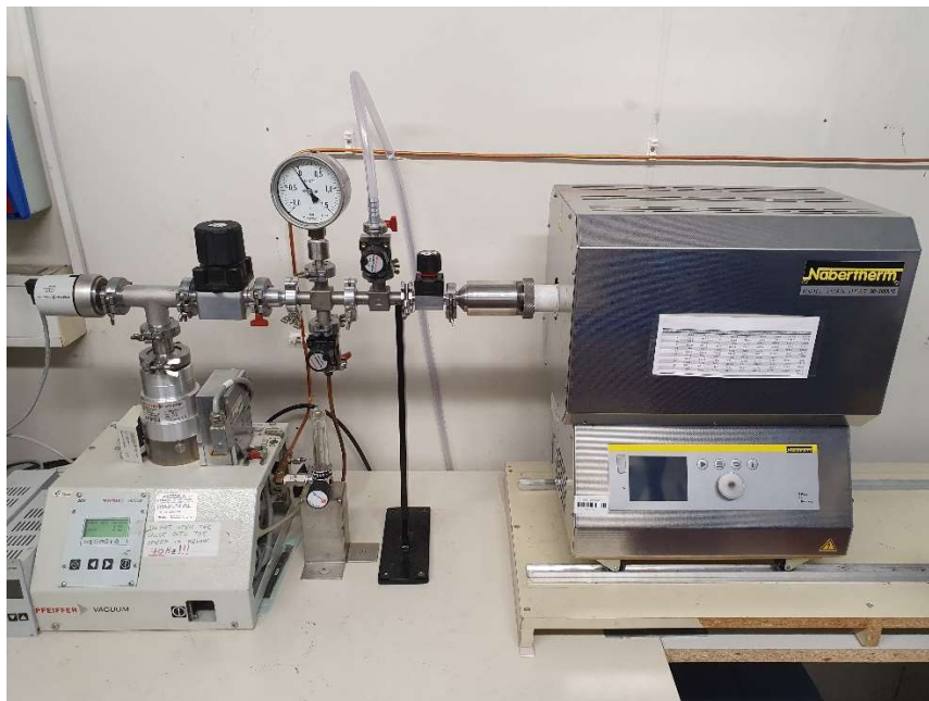
Figure 3.2: Carbolite furnace with vacuum system.
