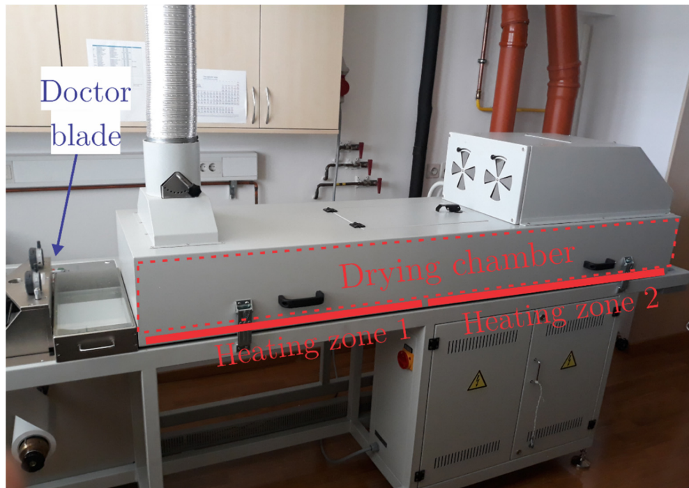
Figure 3.2: Tape caster with the heating zones 1 and 2 marked with a red line.
