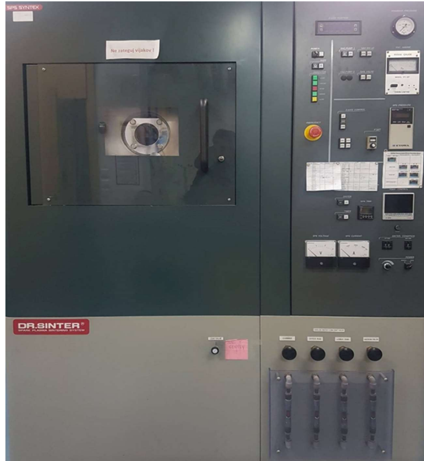
Figure 55: the multipurpose SPS sintering and hot deformation unit.
