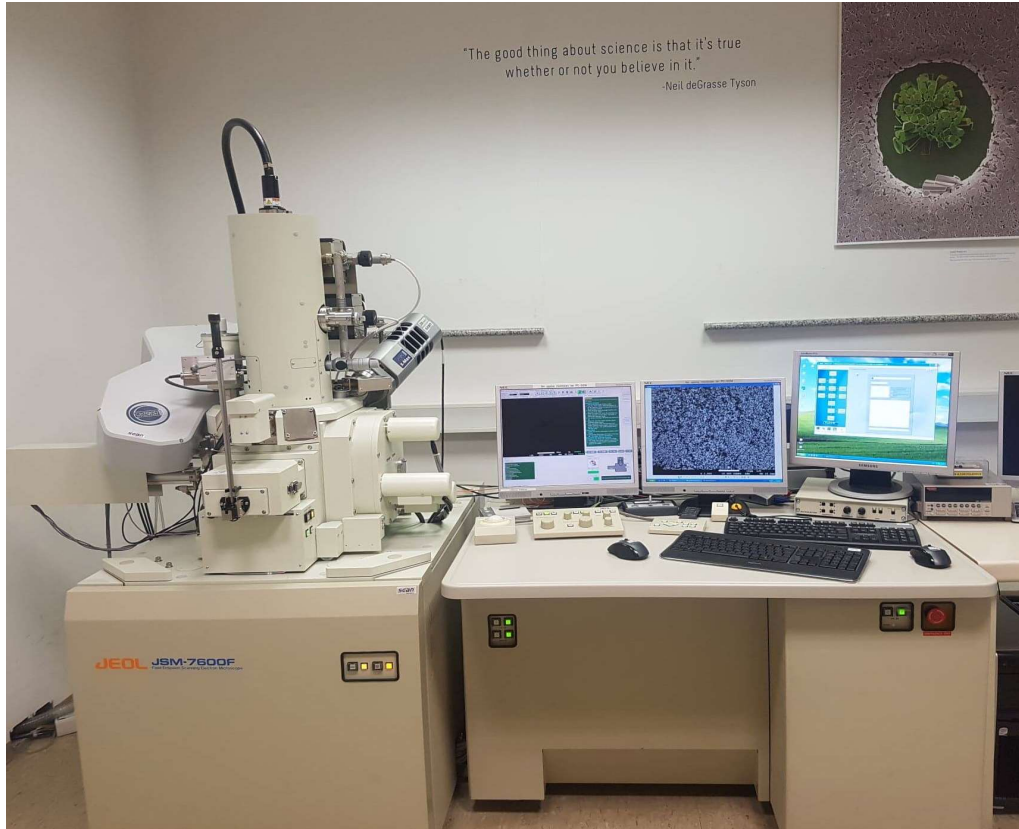
Figure 58: JEOL 7600F FEG-SEM with Oxford Inca 20 mm 2 EDXS detector.
