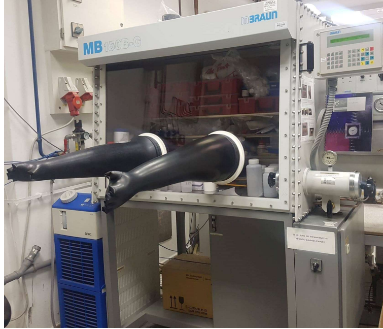
Figure 53: The laboratory scale glove box for handling and storing the powder samples.
