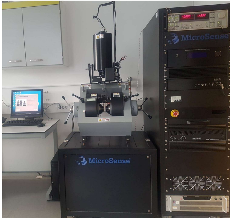
Figure 54: Lakeshore MicroSense vibrating sample magnetometer (VSM) used for determining the magnetic properties of the powder samples.
