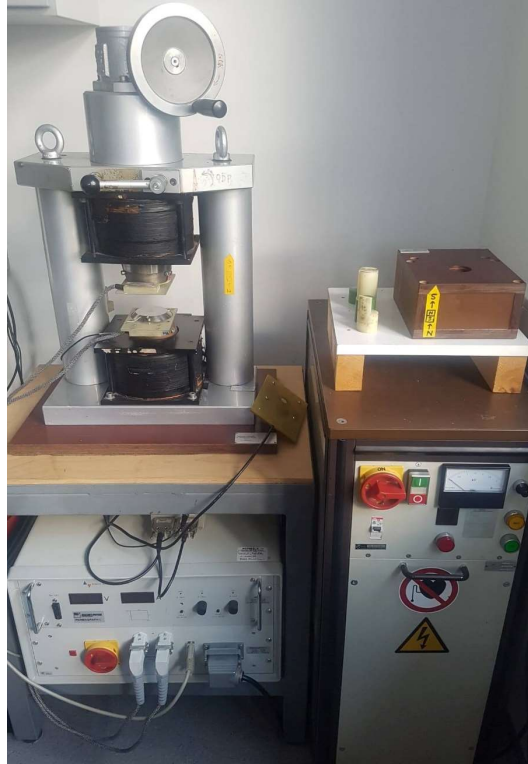
Figure 57: Two electromagnetic coil-based permeameter on the left and 2 T magnetic pulsar on the right.
