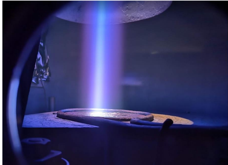
Figure 5.7: Sputtering Ti target with Ar ions in the Sputron deposition unit.
