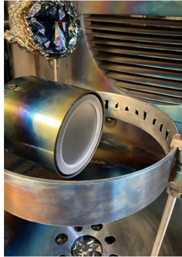
Figure 5.8: Experimental set-up. The samples are positioned in 10^\circ steps on the semicircular holder.
