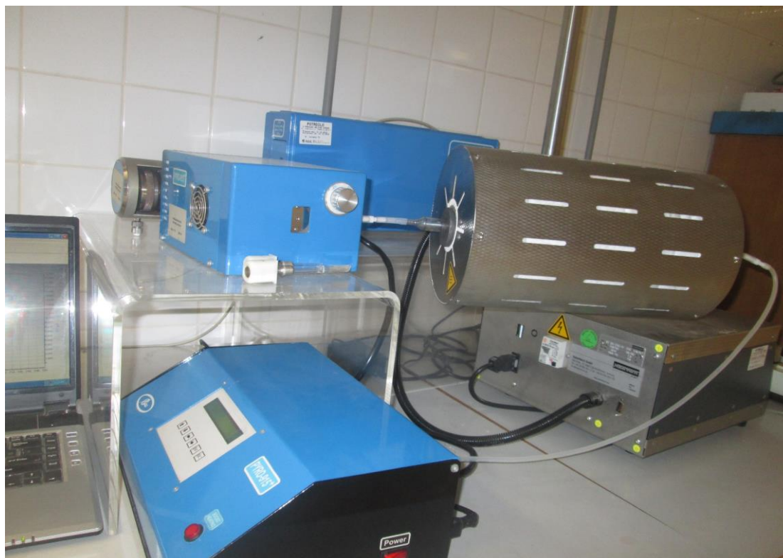
Fig 3.21: Apparatus for thermal fractionation of Hg.
