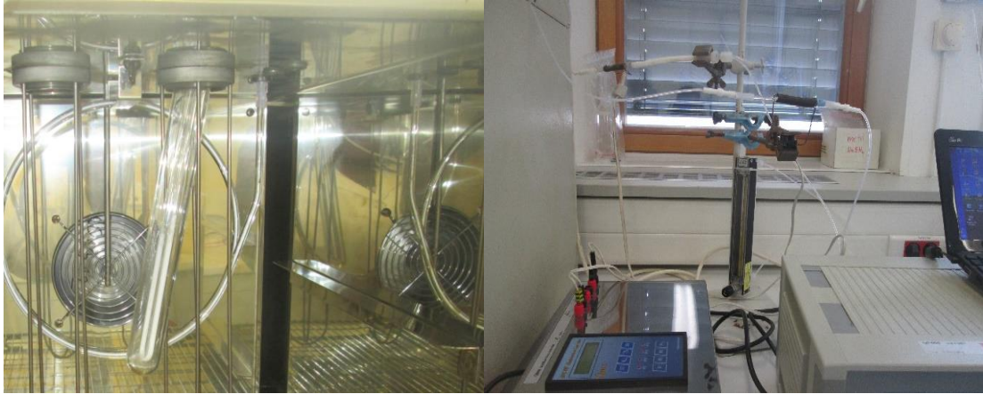
Figure 3.15: Analytical system for thermal desorption, GC-separation of mercury species, pyrolysis and CVAFS detection.
