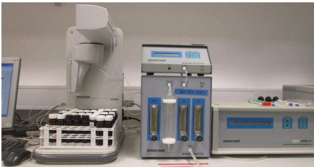
Figure 3.19: Brooksrand “MERX” GC-CVAFS Automated MeHg Analytical System for MeHg measurement in water.
