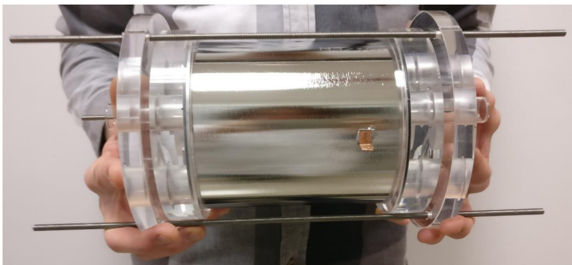
Figure 19: A large-scale photo(electro)catalytic reactor with a volume of app. 1.5 L.
