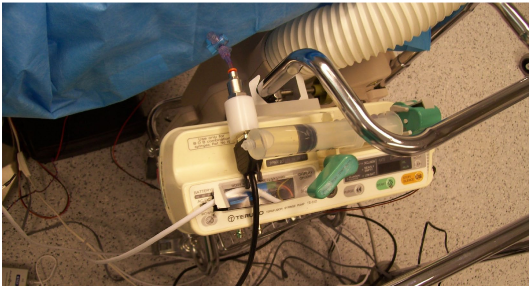
Figure 22 - Syringe pump for automatic balloon inflation
